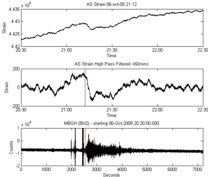
*Figure illustrating the abrupt strain change coincident with the onset of ashventing at Soufriere Hills Volcano. Similar signals have been observed during many venting episodes.*
