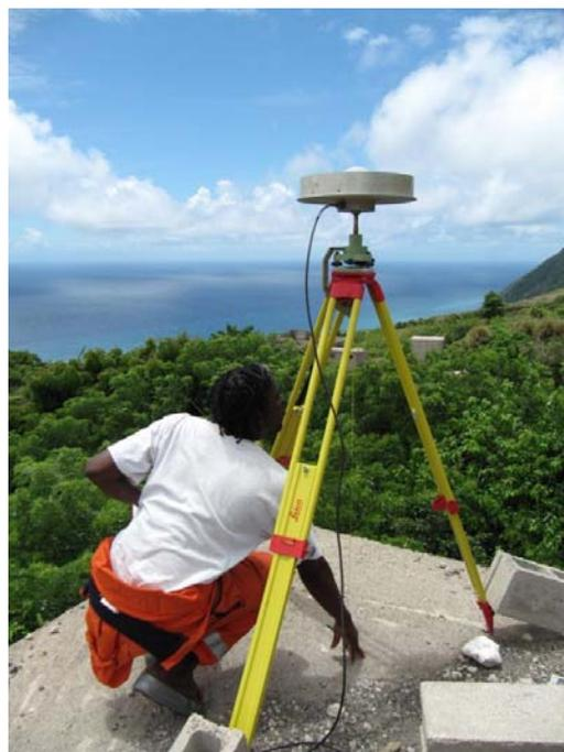
**Above:** Mobile GPS station to monitor ground deformation on the flanks of the volcano.
